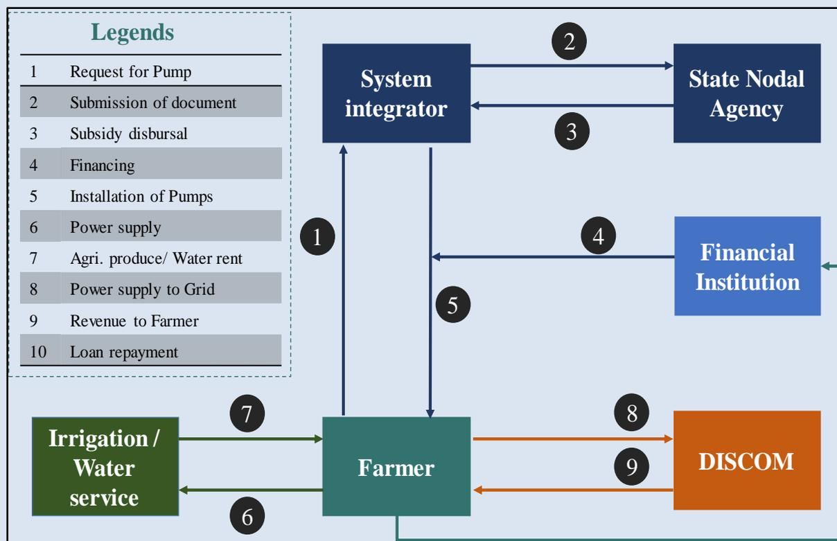
**Figure 10:** Schematic framework of grid-connected SWP
