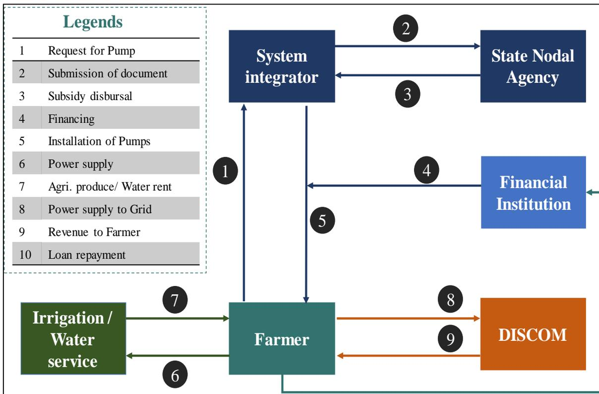
Figure 8 : Schematic framework of grid connected SWP
