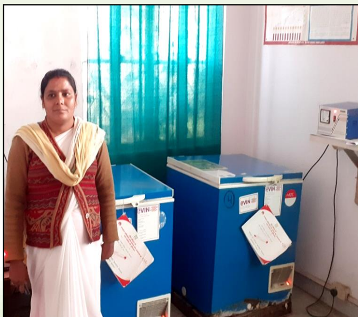
a) ILR connected to eVIN machine b) SIM-enabled temperature logger
